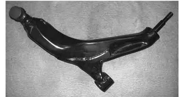
Photo 3 Automotive part applied PRB method and 780 MPa class ERW tube
