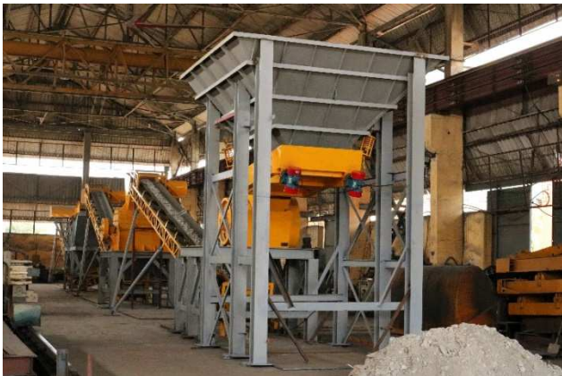
Newly installed crushing machine for recycling CDW in October 2019
