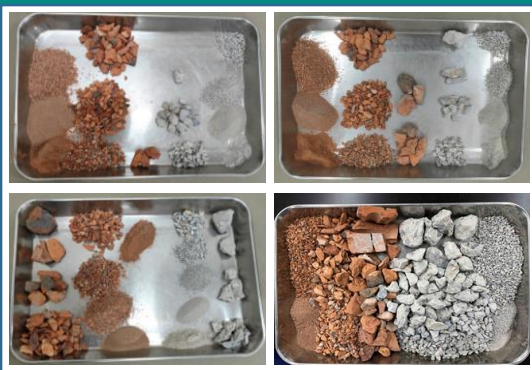
Graded recycled concrete and clay brick aggregates for unbound road base and subbase materials
