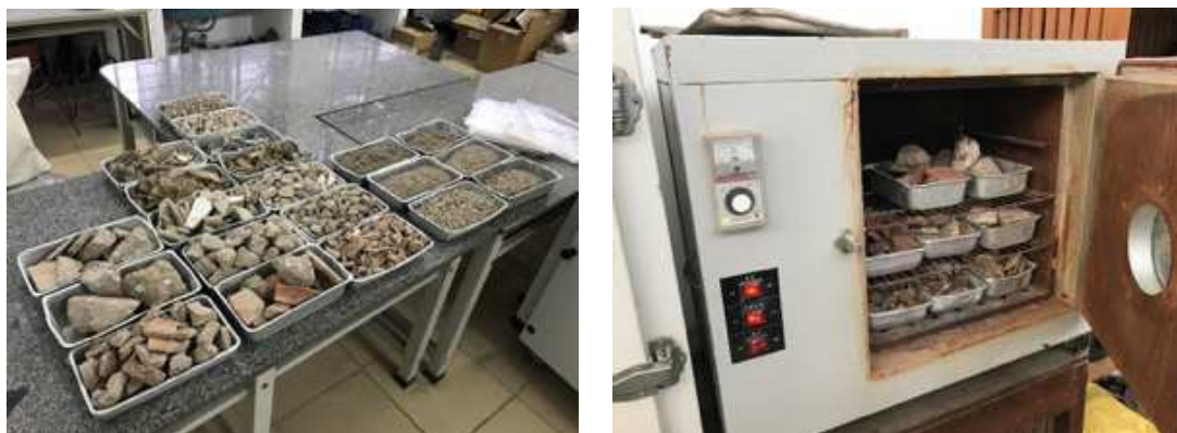
Fig. 10. Water content measurement in the laboratory (oven-drying method).
