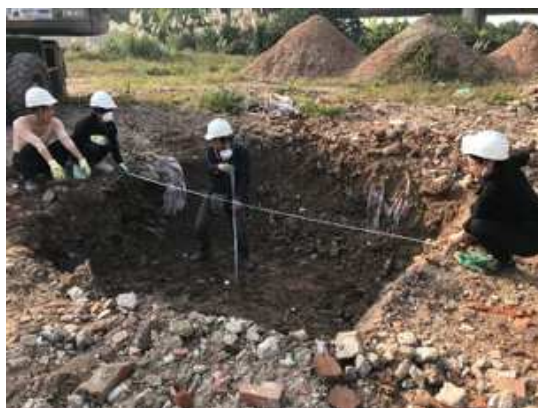
Fig. 13. Sampling pit at Thanh Tri CDW landfill. Photo (left) and scale of pit (right).
