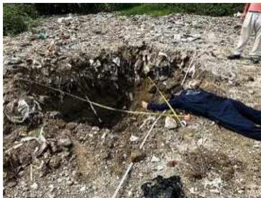
Fig. 18. Sampling pit at Vinh Quynh CDW landfill. Photo (left) and scale of pit (right).
