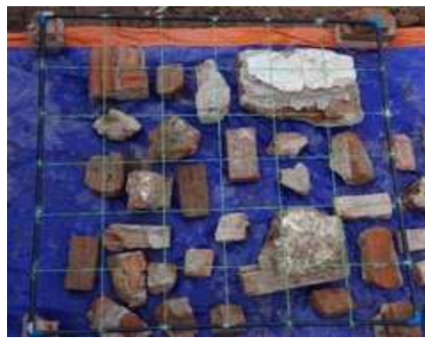
(f) Image analysis (samples >100 mm)
